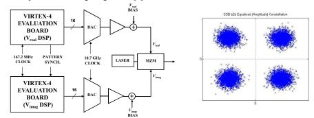
Fig. 1 Left: Transmitter design. Right: Constellation of an 8.35 Gb/s optical OFDM signal generated using the transmitter.
