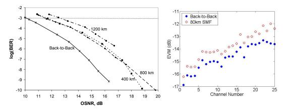
Fig. 2 Left BER versus OSNR for 10.7 Gb/s EPD signals [3], Right: Measured EVM for 8.35 Gb/s OFDM signals
